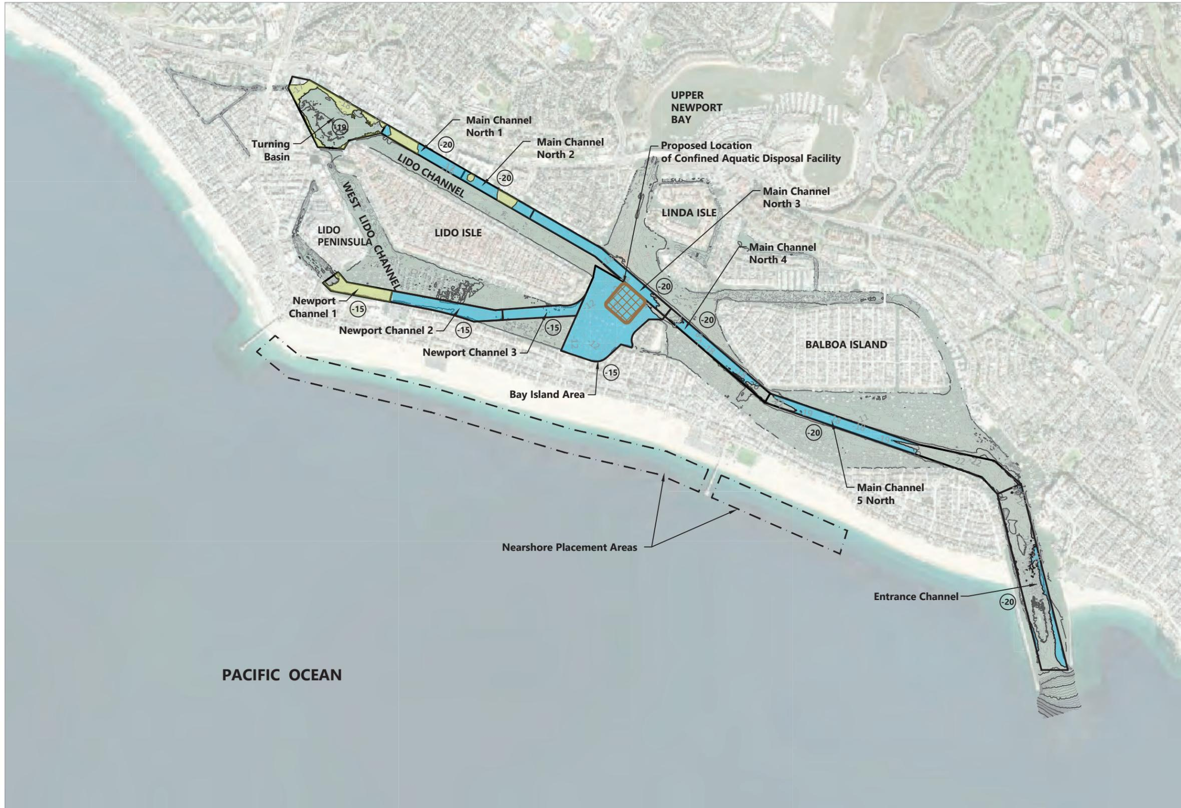
**SOURCE:** Drawing prepared from Bing maps. Bathymetric contours from U.S. Army Corps of Engineers survey dated June 2017. Dredge units from U.S. Army Corps of Engineers.
